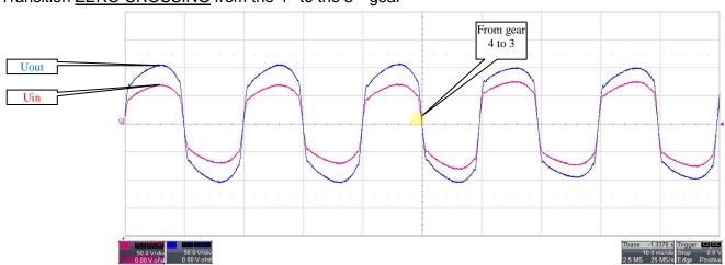
Red – input voltage Blue – output voltage
